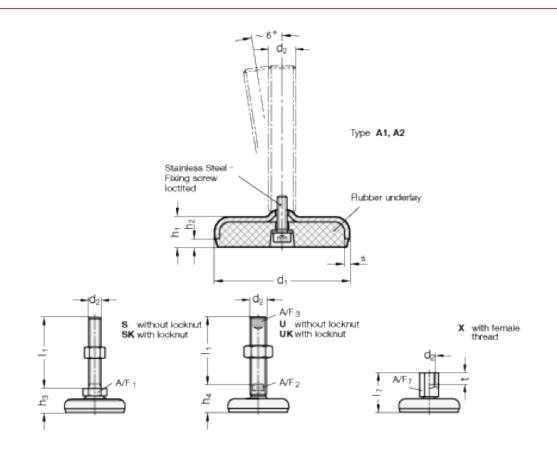
$\begin{array}{l} A/F1 = 17 \\ d1 &= 60 \\ d2 &= M12 \\ h1 &= 16 \\ h2 &= 4 \\ h3 &= 24 \\ l1 &= 80 \\ s &= 3 \end{array}$
